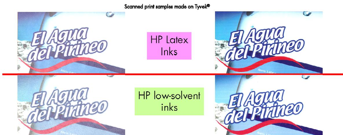
The print samples on the right are made on HP DuPont™ Tyvek® Banner with HP Surface Treatment Technology. Colors are seen to be vivid and saturated with much higher optical density.
