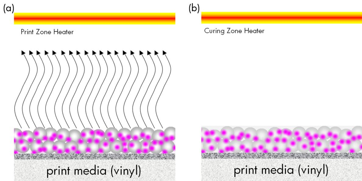
In Figure 3, a continuous latex film encapsulating the pigments has formed on the vinyl surface as the print leaves the Curing Zone. No additional drying of the print is needed because virtually all of the ink vehicle has evaporated. An external print dryer is not needed, and production workflow is improved because prints come out of the printer ready to use, finish (e.g., trim, weld, or laminate), or prepare for shipment.
