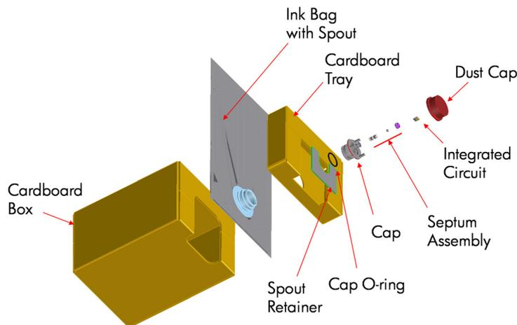
A collapsible Ink Bag inside the box contains the ink and provides vapor and air barriers to minimize changes in ink composition during shipping, storage, and use. A Cap with a Septum Assembly is attached to the Spout
