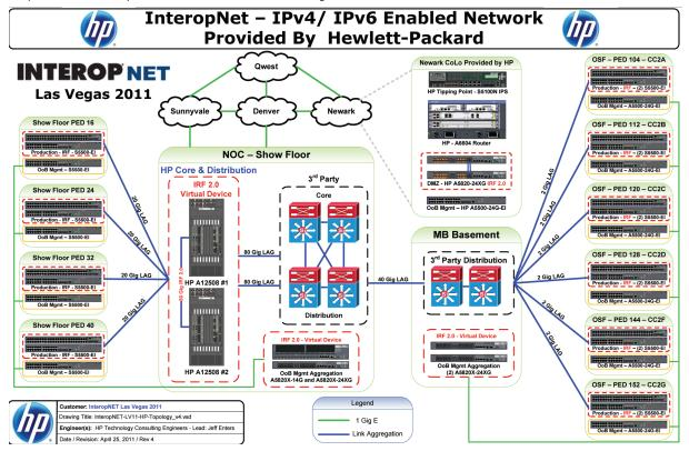
different pedestals, or "peds" scattered across the convention center. These consisted of data closets, cores, initial distribution frames and main distribution frames.
