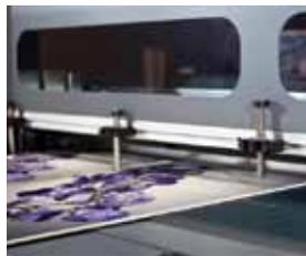
An automatic alignment bar helps you quickly position media, the printer measures its thickness, and an onboard camera detects the position of loaded media.<sup>6</sup> Print up to 4 sheets at once.
