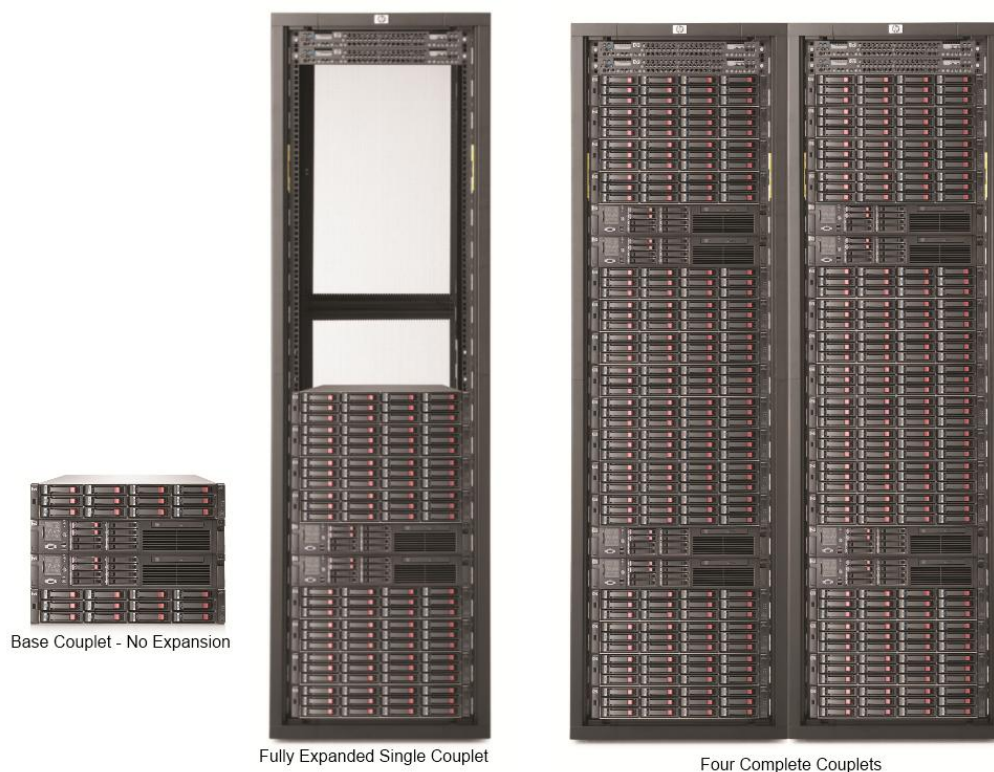
Figure 1: HP B6200 Configurations - This image shows B6200 scalability from the base couplet of two compute and storage nodes, through a fully expanded single couplet in a rack with network switches, to the fully scaled system with four complete couplets.
